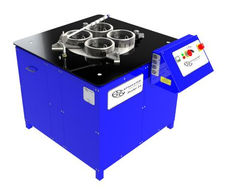
The Lapmaster Wolters Model 24 is the smallest floor standing lapping machine in the range and is ideal for engineering workshops, where flatness and finish are of prime importance. It is equipped with a 610mm diameter serrated lap plate, manufactured from Grade 300 grey cast iron to ISO 185(2005) as standard. Other plates can be supplied on request.
